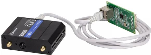
kit ethernet/rj45 + modem 4g + antenne joinon
